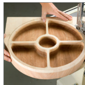
Bandsaw the exterior to final shape.
