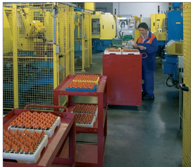
Loading the automated multi-axis CNC sharpening machines.
