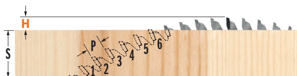
Z_p = 5/6 - CROSSCUT, CHIPBOARD, MDF, PLYWOOD, LAMINATE, PLASTIC
