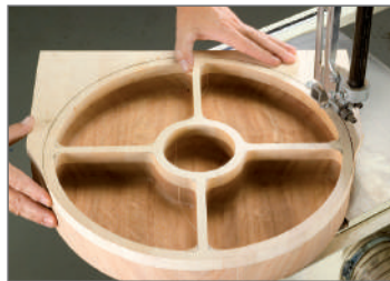
Bandsaw the exterior to final shape.
