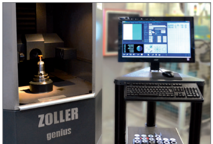
CMT's fully automatic measuring system.
