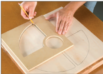
Trace the templates onto the bowl blank.
