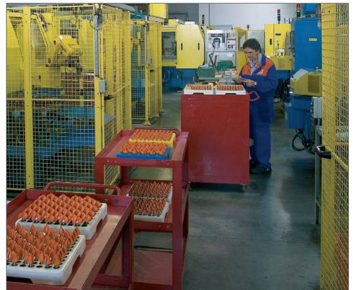
Loading the automated multi-axis CNC sharpening machines.
